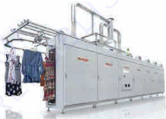
Fig: Tunnel finisher
