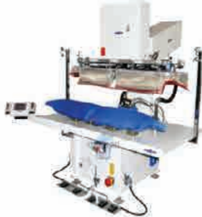
Fig: Cannon press for jacket pressing
